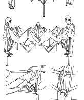
3. Each partner should then grasp the bottom of the middle frame section(cross beams) where it forms diamond. Lift slightly and slowly walk backward until the frame is fully extended. Be careful not to pinch your finger or pull backward too hard as this may result in the bending of cross beams.
