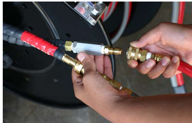
The Spray Gun Quick Connect Plugs attach to the Spray Gun Quick Connect Sockets.
