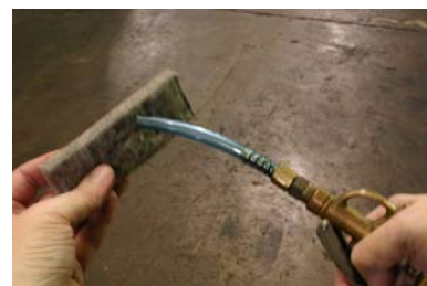
Cleaning the compressor air filter with compressed air.
