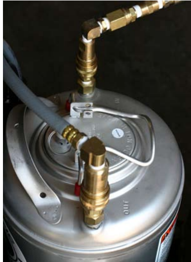
The Tank Quick Connects connect the tank to the incoming airline and outgoing liquid line.
