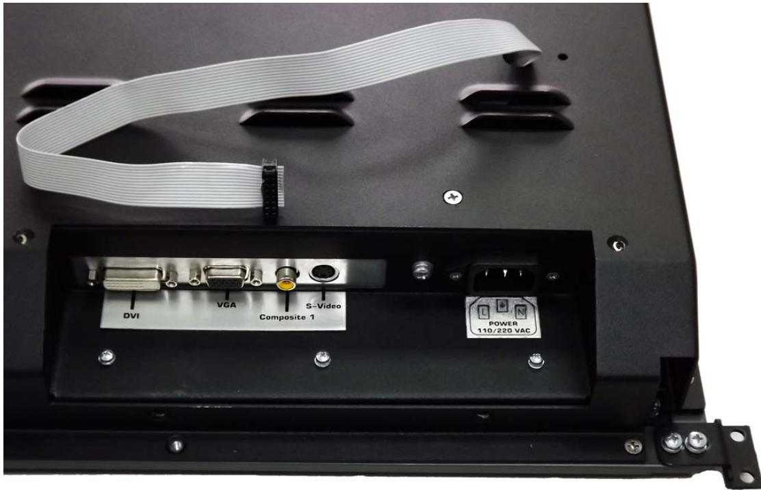
Figure 14. Location of connectors and control cable in LCD display
