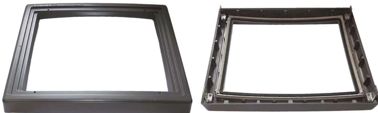
Figure 4. CRT frame view (removed from radar rack)
