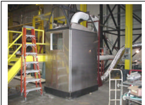
Total Enclosure Test Stand
