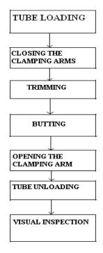
**Tube loading:** this is the first step in splicing operation in which the tube is loaded manually by the operator between the two jaws, leaving some portion of the tube (usually 5 to 10 mm) to project from the two ends of the jaws, which is trimmed leaving a small length of the tube from the jaw ends (0.5 to 1mm) called overhang for facilitating butting operation.
