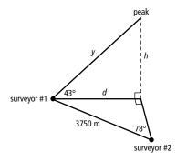
a) Find the distance d, in metres, from surveyor #1 to a point directly under the peak:
