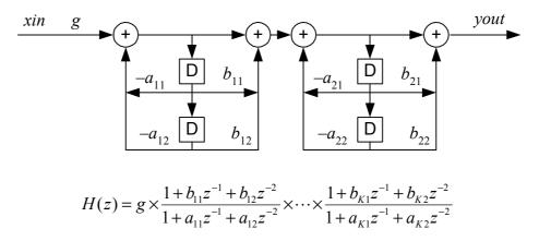
Note that you only need a single gain coefficient, g, for the whole filter and do not need individual  $b_0$  coefficients for each stage. You may find it easiest to have four separate coefficient arrays for the  $a_{*1}, a_{*2}, b_{*1}, b_{*2}$  values. In MATLAB, you can convert a direct-form filter into cascaded second-order sections using the function tf2sos(). Verify that your bandpass filter works correctly.
