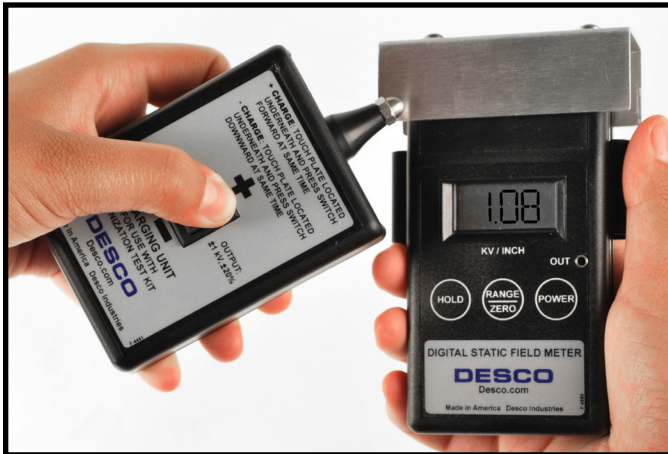
Figure 8. Taking decay measurements
