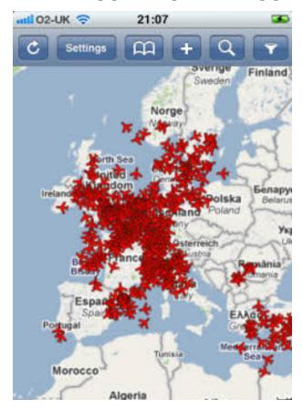
Plane Finder, which can be downloaded for only £2.99, works by picking up ADS-B plane feeds used by all commercial planes to transmit their name, position, destination and lots more. This technology is actually faster than radar and is used in some places for air traffic control and navigation.
