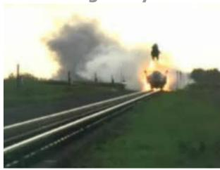
No, not the long awaited new Kitfox ejector seat. This one is for the F 35 Lightning, tested on a track at speeds of up to 600 mph. You can see film of it below, and yes, it was a dummy in there, this time.
