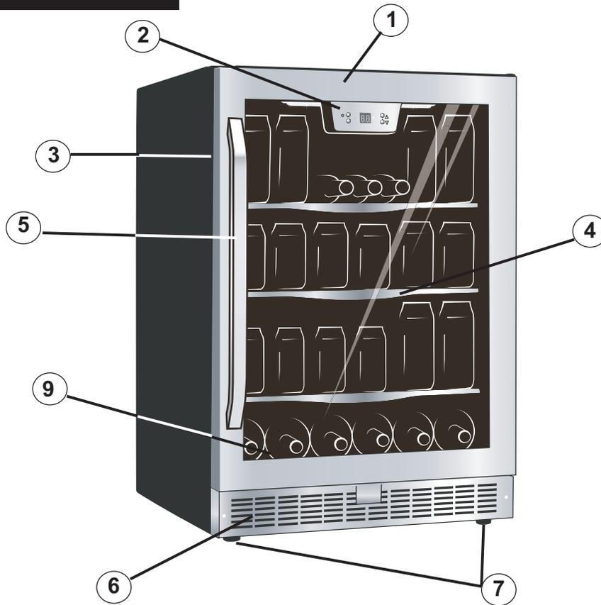
**1. Tempered Glass Door:** Tinted for UV protection while still allowing for easy interior viewing.
