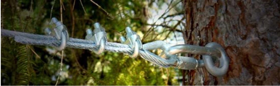
Figure 42: An Actual Cable with Cable Clamps and Thimble
