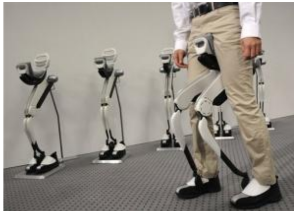
Figure 9: Honda's Assist Walking Device
