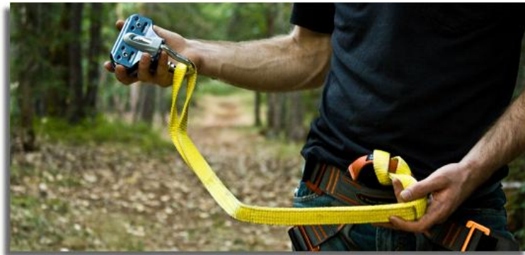
Figure 51: Lanyard Connected to Pulley via Carabiner and Tie Point in Harness
