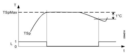
TSpMax Storage tank temp max (operating line 5051)
