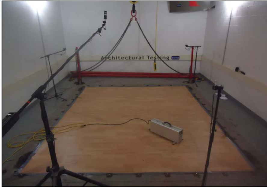
Source Room View of Test Specimen Installation
