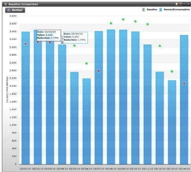
The baseline can be plotted as a line, dashed line, or color-coded bubbles, as seen in the example above.
