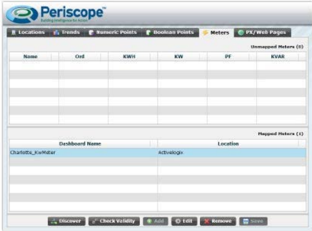
Be sure to map the newly created meter within Periscope's configuration browser. Here the user can give the meter a name and assign it to a location.
