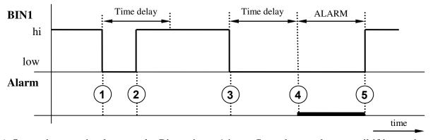
A figure shows a simple example. Binary input 1 is configured to send an e-mail if input change state from high to low (lower edge). At point 1 a binary input was opened. Because at point 2 input was closed before the time delay expired, alarm was not set. At point 3 was input opened again. At point 4 the time delay expires and at this moment e-mail, SNMP traps are sent. The alarm lasted to point 5, where the input was closed.
