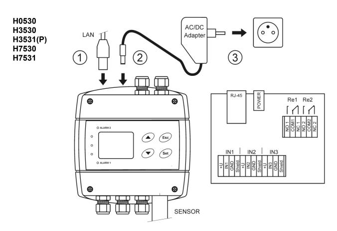
Binary inputs are not galvanic isolated, connection terminals +U are internally connected to the device power supply (ie. the +U terminals provide the same voltage level as power supply).
