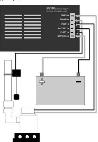
**BATTERY:** The battery should be placed inside its protective battery box before being connected to the charger unit. Make sure that the charger unit is not plugged into the wall outlet.
