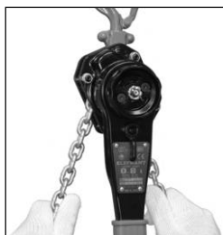
3) You can adjust the length of load chain by pulling it.
