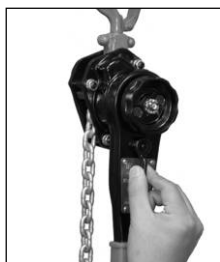
1) Set the selector lever to "N" position.
