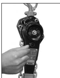
4) Set the selector lever to "UP" position.
