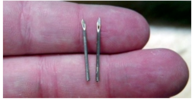
Fig. 3. Two injection needles found in beef carcasses.
