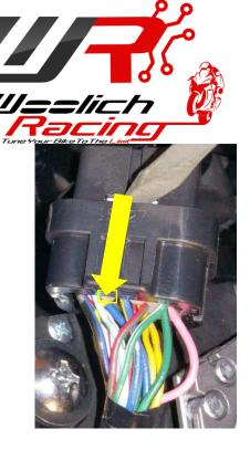
7. Use a pick or scribe to pull the white plastic dust plug out the backside of the connector. Or if preferred, a small paper clip can be unwound and inserted in the connector side of the plug and used to push down and push the plug out the backside of the connector. Remove and discard of plug.
