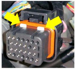
Use the flat head screwdriver to press them down flat; this locks the pins into place in the connector
