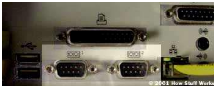
Two serial ports on the back of a PC
