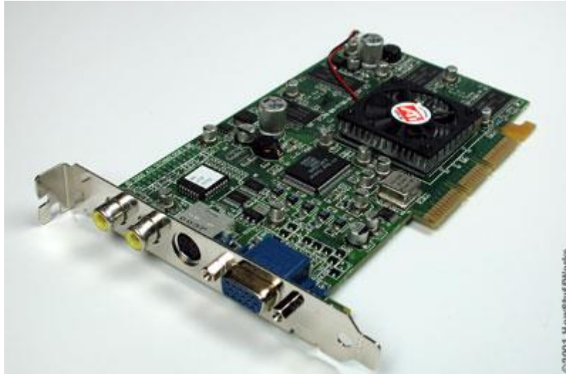
Typical example of an AGP-based graphics card
