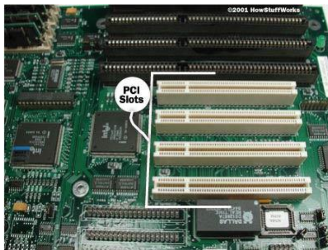
This motherboard has four PCI slots.
