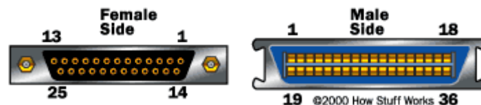
Female side and male side of a parallel port
