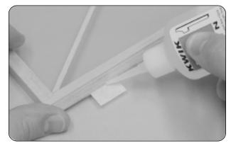
□ Center each hinge within its precut slot in both ailerons. If you can't push the hinge in halfway, carefully cut the slot deeper using a modeling knife.
