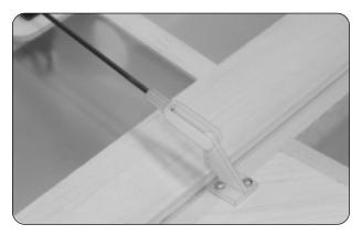
□ Thread one clevis onto the pushrod wire and snap it into the **outermost hole** in the control horn.
