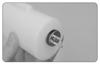
□ When satisfied with the alignment, tighten the machine screw until the rubber stopper expands and seals the fuel tank opening.
