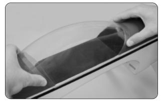
□ Set the canopy onto the fuselage and align it. The canopy should be centered over the middle of the fuselage when looking from the front and it should be centered over the cockpit area when looking from the side.
