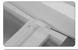
□ Thread the clevises onto the pushrod wires and snap them into the **outermost hole** in the control horns.
