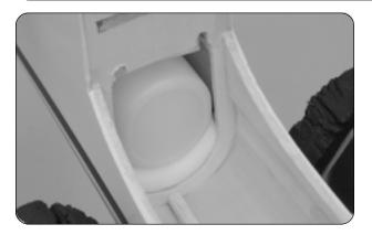
□ Cut and install several pieces of foam rubber between the bottom of the fuel tank and the top of the fuel tank support platform, and between top of the fuel tank and the top of the fuselage, to wedge the fuel tank securely into place.
