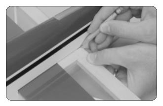
□ When you're satisfied with the alignment of the trailing edge, draw a mark on each side of the stabilizer (at the trailing edge) where it meets the fuselage sides.
