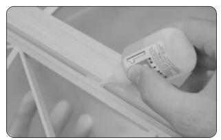
□ While holding the aileron tight against the wing panel, pivot the aileron down about 45° and apply 5-6 drops of thin C/A to the exposed area of each hinge. Turn the wing panel over and repeat for the other side of the hinges.
