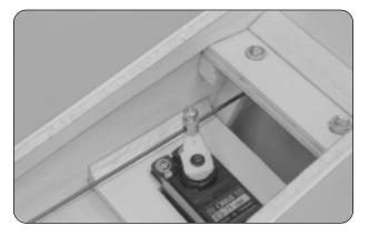
□ After making sure that the carburetor is in the fully closed position, angle the servo horn back about 45° from center and attach it to the servo output shaft. The servo connector should be facing the side of the fuselage.
