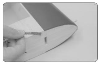
□ Using a modeling knife, cut away and remove the excess covering material that overlaps onto the root ribs of each wing panel, leaving about 1/16" overlapped so it does not pull away.
