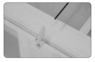
$\Box$  Mount the control horn to the aileron, directly behind the pushrod wire, using two M2 x 15 machine screws. Make sure that the control horn is parallel to the hinge line and that the clevis attachment holes are over the hinge line.
