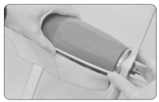
□ With the cowling temporarily in place, secure your spinner backplate to the engine's crankshaft.
