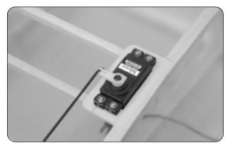
□ Center the aileron servo and install the servo arm assembly making sure that the servo arm is centered and points toward the wing tip.
