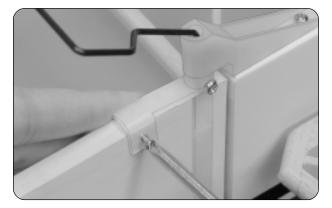
□ While holding the tiller arm firmly against the bottom of the rudder, drill a 5/64" diameter pilot hole through both sides of the nylon clasp and through the rudder.
