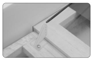
□ Position one nylon control horn onto the bottom of one elevator half, aligning the centerline of the control horn with the pushrod wire. The centerline of the control horn should be approximately 3/4" out from the side of the fuselage.
