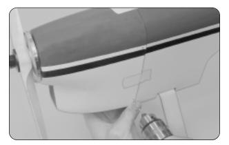
□ With the cowling held firmly in place, drill 5/64" diameter pilot holes into the cowling and through the fuselage for the four wood screws. Locate two holes on each side of the cowling, 1/4" in front of the back edge of the cowling. One hole should be 1/2" up from the bottom of the cowling, and the other hole should be just below the cowling's upper radius.
