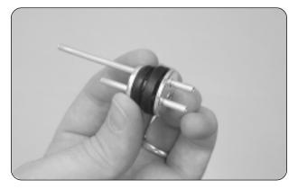
□ Push the two aluminum tubes through the rubber stopper. Slide the large diameter metal plate over the tubes at the front of the stopper and slide the small diameter metal plate over the tubes at the rear of the stopper.
