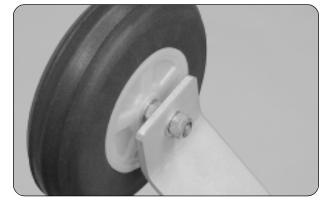
□ Slide the axle assembly through the predrilled hole in the main gear strut and secure it into place using one M4 flat washer and one M4 lock nut. Tighten the lock nut firmly while holding the inner lock nut in place with a pair of needle nose pliers.
