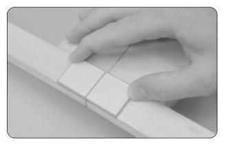
□ Using thick C/A, glue the wing-screw doubler to the **bottom** of the wing, making sure that the centerline you drew lines up with the centerline of the wing, and that the back of the doubler is even with the trailing edge of the wing.
