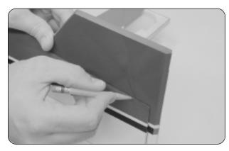
□ While holding the vertical stabilizer firmly in place, use a pencil to draw a line on each side of the stabilizer where it meets the top of the fuselage.
