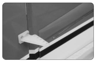
□ Use a couple of pieces of masking tape to hold the rudder centered.
