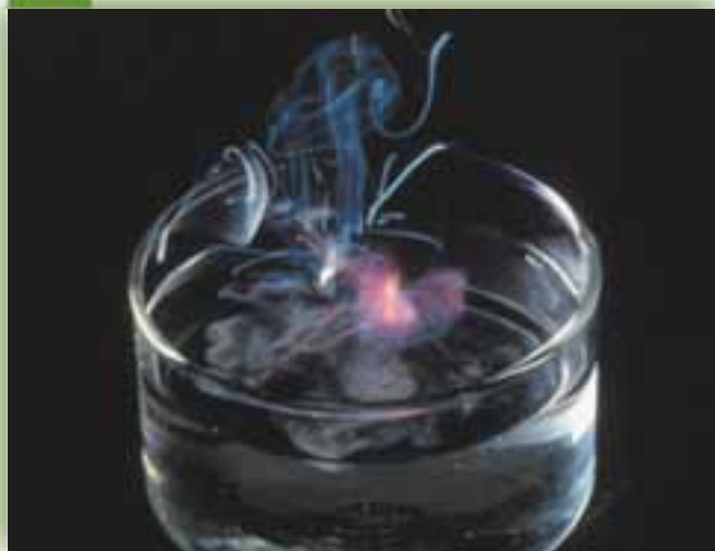
Fig 1.5.7 Potassium in water. Reactions become more violent as we move down Group I.
