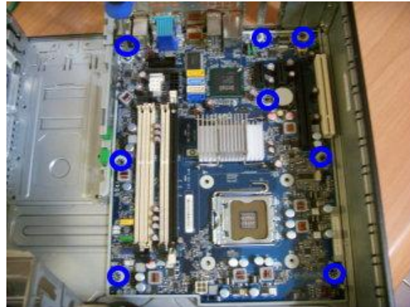
Figure 22: Release PCA 8 screws by wresting screw with screw driver
