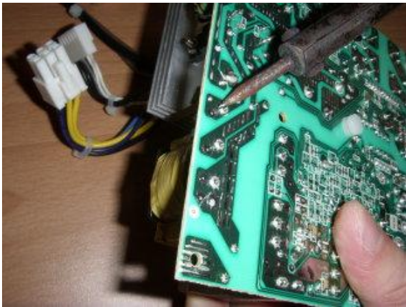
Figure 33 Remove electrical capacitors
