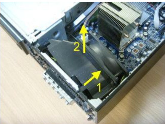
Figure 9 : Remove fan and fan holder from chassis
