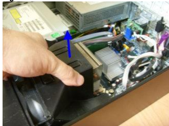
Figure 6: Release Fan duct
