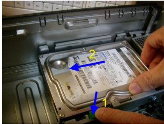
Figure 20: Release HDD Press HDD latch and push HDD toward Front side.
