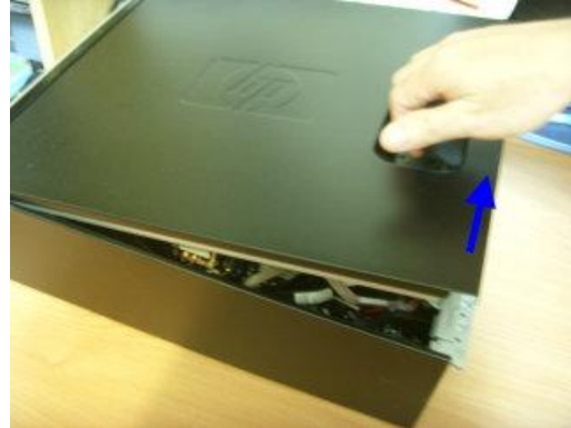
Figure 2: Rise access panel Press front panel clip
