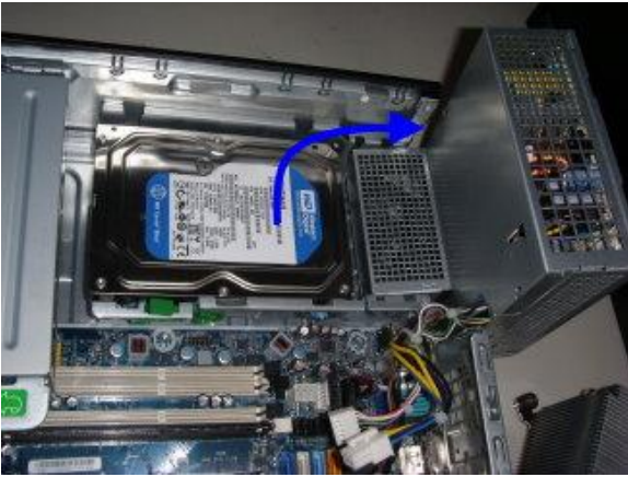
Figure 21: Remove PSU from Chassis
