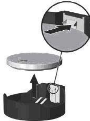
Figure 24: Press Battery holder and Pull battery
