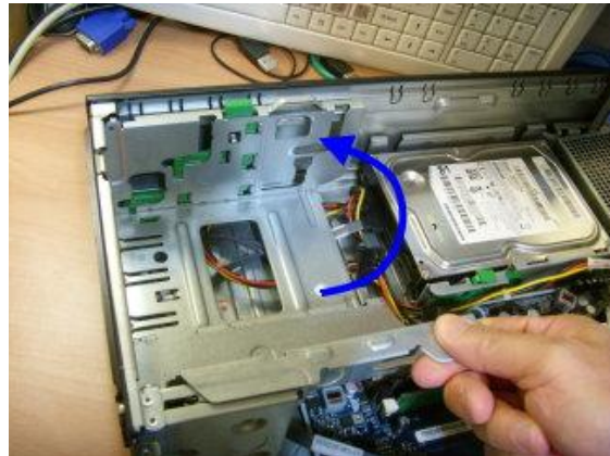
Figure 18: Rotate ODD cable to vertical
