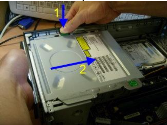
Figure 17: Release ODD from ODD cage Press ODD latch and push ODD toward PSU.
