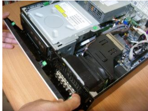
Figure 4: Release the front bezel. Rotate the bezel outward to remove it from the chassis
