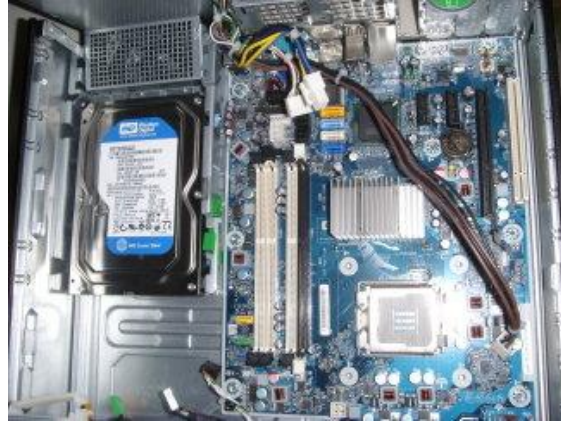
Figure 16: Remove all internal cable from PCA
