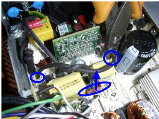
Figure 29: Cut PSU PCA wire (2) and disconnect Fan connector
