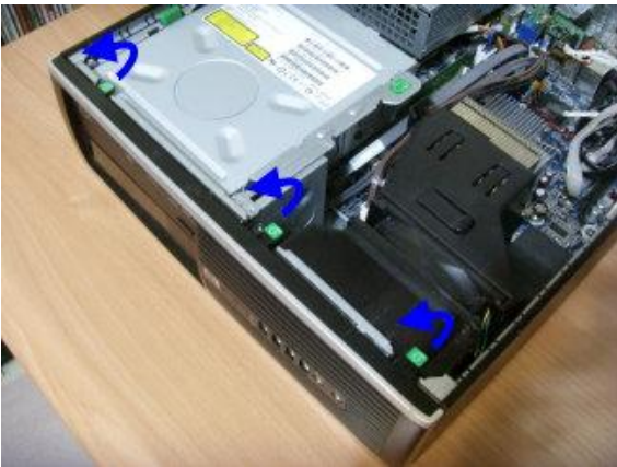
Figure 5: Remove all cable from cable clamp
