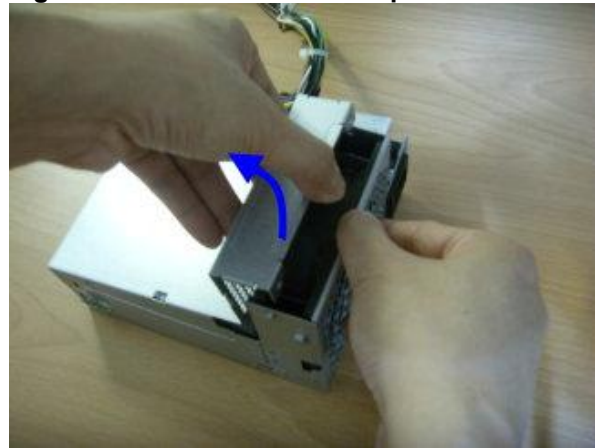
Figure 28: Remove PSU the top of case
