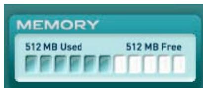
This bar is a visual representation of how much of the memory in the CRAMMER handheld is being used, and how much is available for additional files. The gauge is only active when the CRAMMER handheld is connected and turned on. The CRAMMER handheld has 1 GB of memory available. You can add as many components to your CRAMMER handheld as can be stored in that amount of space. If the memory on the CRAMMER handheld is full, you will need to remove at least one file in order to add additional files.
