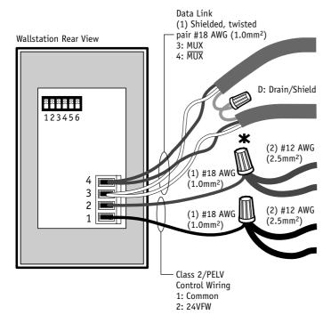
Make connections inside the wallbox. Or in a switchbox or junction box with a maximum wire length of 8 feet (2.5m) from the link to the Wallstation.
