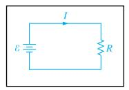
A single resistor *R* is connected to a battery as shown above. The current is *I* and the power dissipated as heat is P. The circuit is changed by doubling the emf & of the battery while *R* is kept constant.
