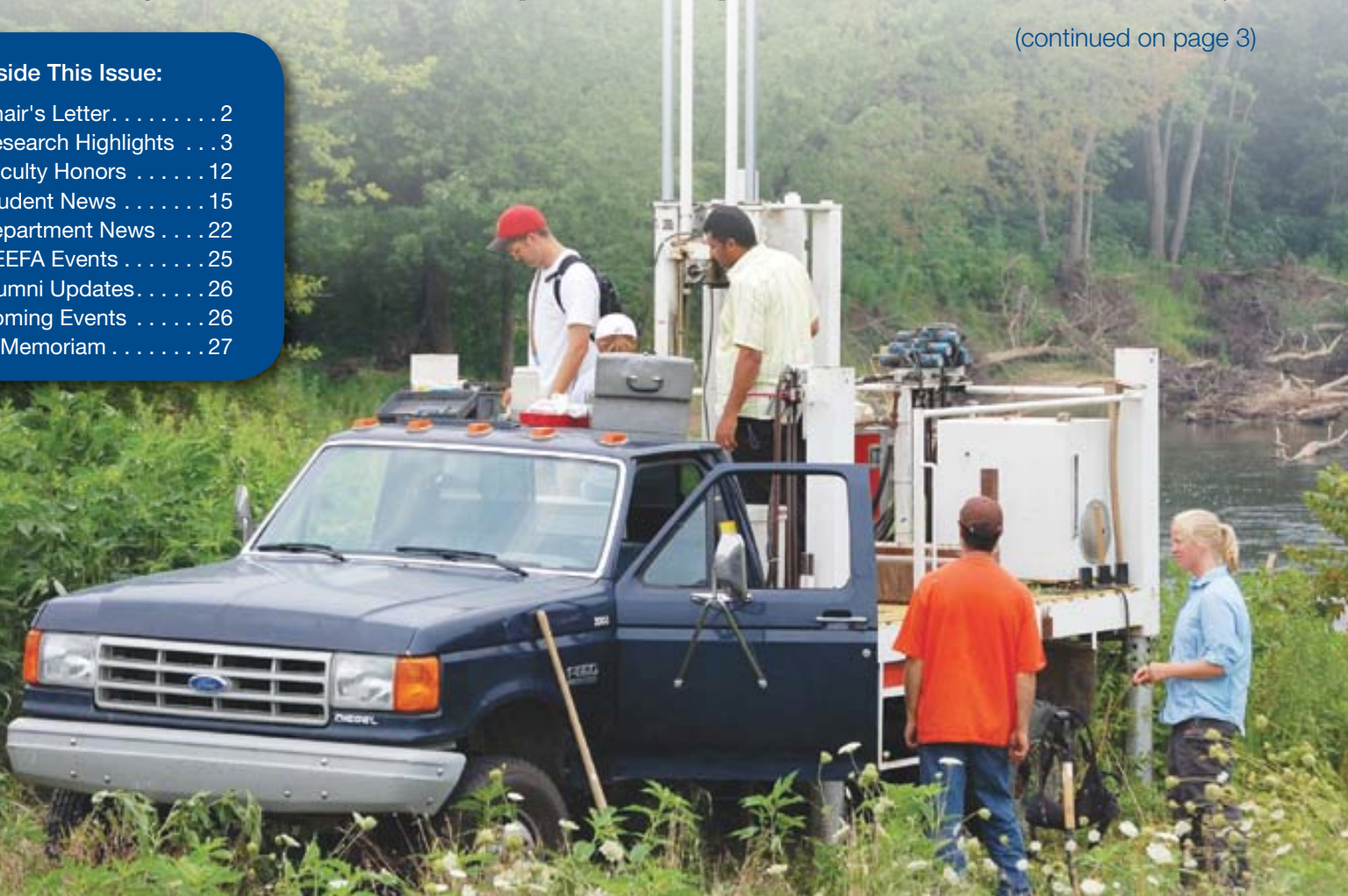
The geotechnical group operates a field vehicle for research and for development of new in-situ soil testing equipment and procedures. Students can augment classroom instruction and laboratory testing with advanced field studies.
