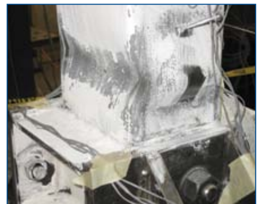
A white coating is used to help visualize the deformations in the HSS members during testing.
