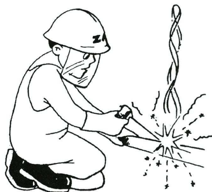
Figure 3: Fumes from welding workks are very toxic in a confined space.
