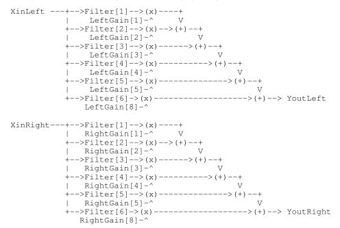
The advantage of this approach is that the filters (filter coefficients) don't change, only the gain adjustment multiplication factor changes.
