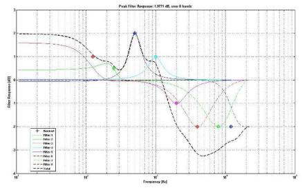
The advantage of cascading filters is that the filters don't need to waste effort attenuating out-of-band frequency but instead just adjust the frequency response by adding gain to increase the signal or attenuation to decrease the signal. The disadvantage is that the size of each filter's manipulation must be known to design the filter's coefficients. So it is not possible to adjust the cascade's overall frequency response once the coefficients are loaded into firmware.
