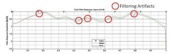
Note there are filtering artifacts not only at the peak of the filter's gain, but at other frequencies as well. The takeaway: *Never* overdrive the filters!
