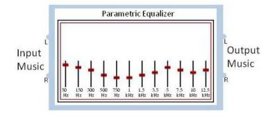
Examining the filtering structure of a parametric equalizer reveals why the signal strength display is missing. As seen below, parametric equalization is accomplished by a chain of back-to-back filters, with each filter having 0 dB (unity) gain outside of specified frequency range.
