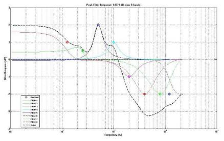
The takeaway from this is that some types of parametric filters, especially those centered at low frequencies, are very sensitive to coefficient rounding. But since using 32 bit filters for an 8-filter setup is only 23% more computationally expensive than the same setup with 16-bit filters, it is usually not necessary to design and use 16-bit filters.
