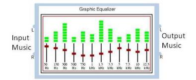
In this example, frequency bands are centered at 50 Hz, 150 Hz, 300 Hz, ..., 10 KHz, and 12.5 KHz. Signal strength is plotted for each frequency band by a stack of green bars, more bars meaning a stronger signal. Below each stack of green bars is a slider that is used to adjust the filter gain for each band, which is centered at the frequency shown. Moving the red tab up increases filter gain, increasing signal strength. Moving the red tab down decreases filter gain, decreasing signal strength.
