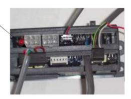
6). Locate the machine MDB harness and disconnect the coin mech/note loader harness from the machine MDB harness. Remove the "Y" harness that connects the coin mech and the note loader together. You will not be using this harness.
