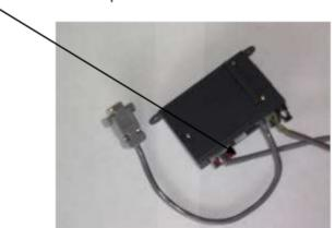
4). Locate the machines MDB harness and disconnect the coin mech/note loader harness from the machines MDB harness.
