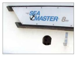
I started by cutting a hole in the superstructure for the flush mounted plug, I was extremely lucky to miss an internal piece of wood by 1mm. I then fitted the fuse box, then the 13 amp
