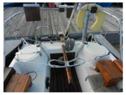
worked extremely well throughout the season and show no sign of wear, they also ease the wear on the bolt hole in the centre-plate. The centre-plate retaining bolt was released, regreased and retightened, this will be done on an annual basis ensuring that the centre-plate will always be able to be removed if required.
