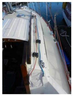
reefing system to flatten the sail adequately, and ensuring that all the lines brought back to the cockpit worked efficiently. I've supplied pictures of the line layout port and starboard of the offset hatch which also show the arrangement at the base of the mast.
