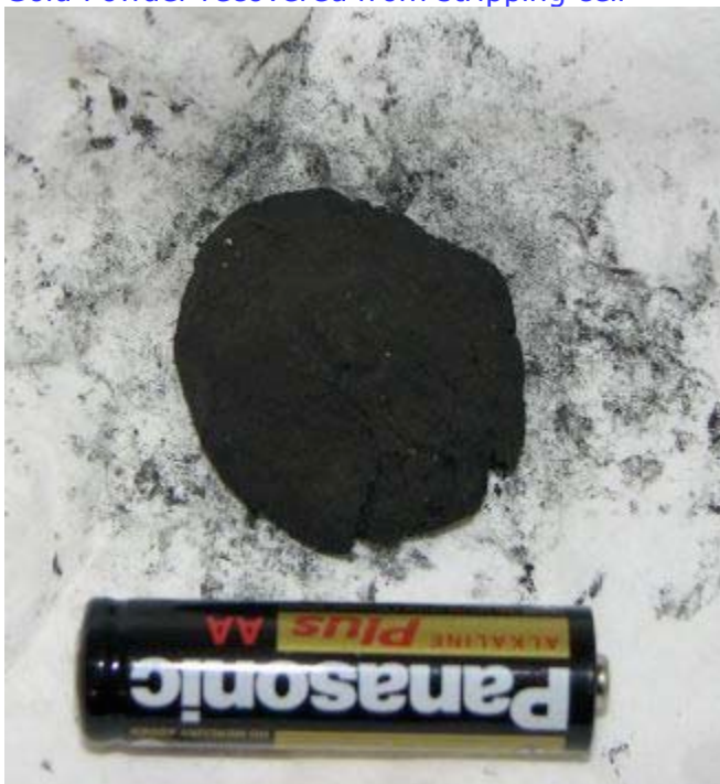
Gold Powder recovered from stripping cell
