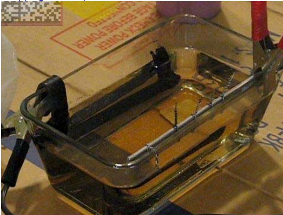
Stripping cell for plated items.
