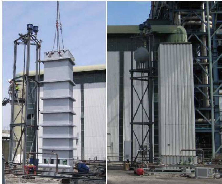
Figure 19. PCM test module at the test site; left: delivery of the module; right: insulated module [14]
