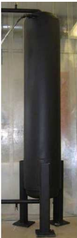
Figure 26. \text{NaNO}_3 PCM Storage Test Module [27].
