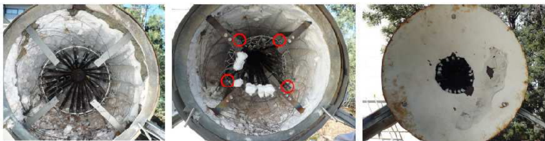
Figure 38. Three receiver configurations viewed looking in to the aperture. Left: Receiver with a 7.5° half cone angle (front shield removed). The indents in the wall insulation indicate the position of the tubes in the frustum with a 17.° half cone angle. Centre: Receiver in a frustum with base radius 77 mm (front shield removed). Right: Receiver as a frustum with base radius 77 mm, but with minimal insulation on feeder tubes (front shield in place).
