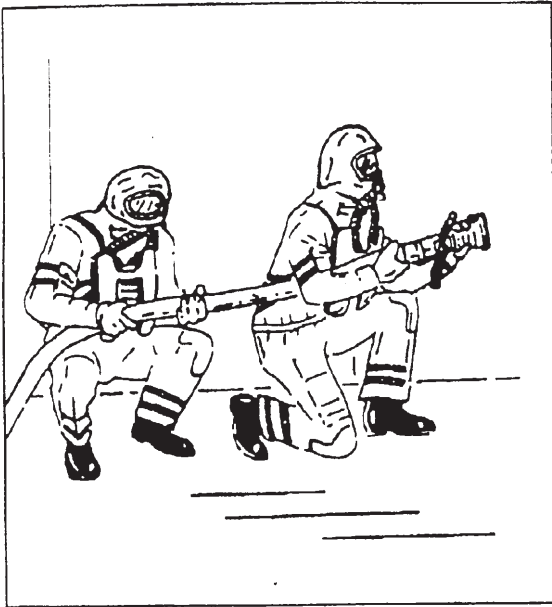
E. UNDER THE ARM, NOT USING PISTOL GRIP GRASPING THE PATTERN SHROUD.
