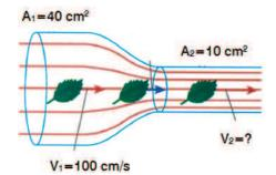
What would be the flow speed in the smaller section?
