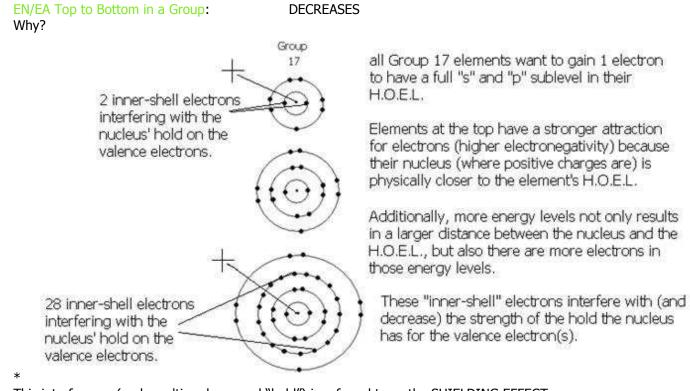
This interference (and resulting decreased "hold") is referred to as the SHIELDING EFFECT.
