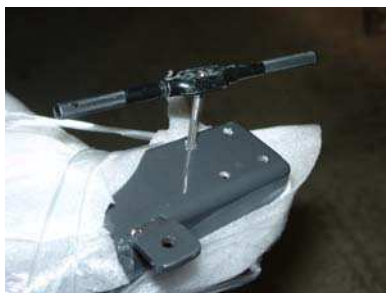
Tire carrier latch installed on tire carrier.
