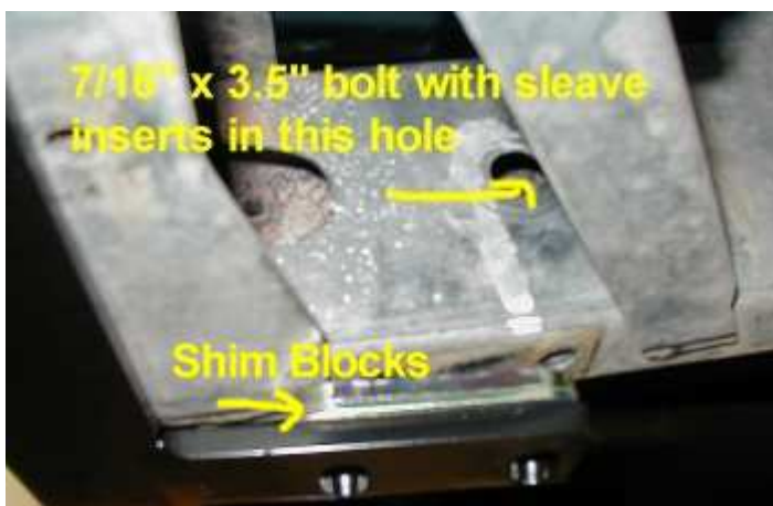
Inside view of rear bumper bracket and frame rail showing location of side mount hole and shim blocks installed.
