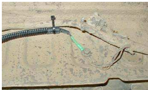
Ground Wire Connected
