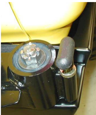
Tire Carrier installed on bumper.
