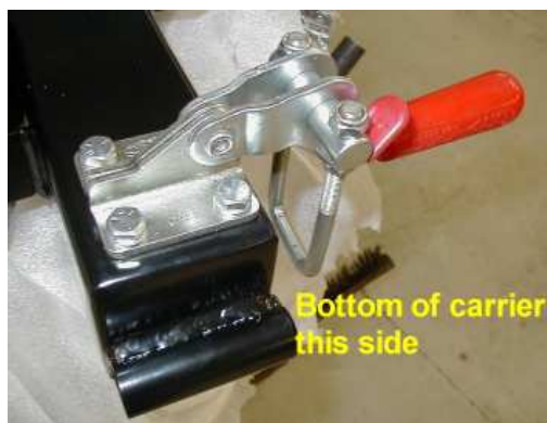
Tire carrier latch installed on tire carrier.
