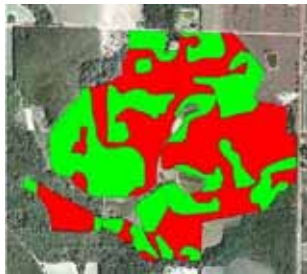
The photo on the left shows the soil electrical conductivity of a field measured by a Veris machine. The zones shift from sandy soils (light red) to heavier soils (dark red). The photo on the right shows where Telone® II soil fumigant will be applied in the same field. Areas in red are low EC zones and will receive treatment. Areas in green are high EC zones and will not receive treatment.
