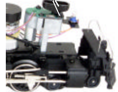
Figure 6. Smoke Unit Inspection Cover
