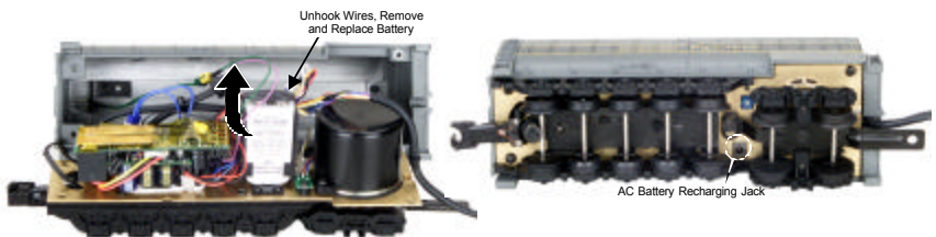
Figure 9. Replacing the Battery and the Proto-Sonnd 2.0 Battery Recharging Jack.
