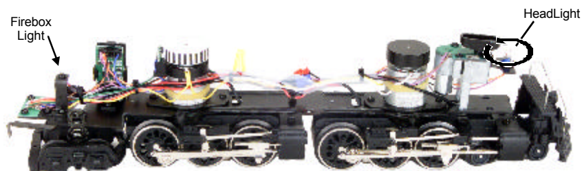
Figure 8. Replacing the Headlight and the Fire Box Light
