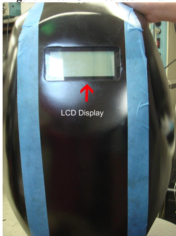
Figure B.10: LCD Mounted in Tank
