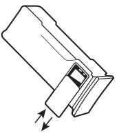
pack. The orientation of the battery contacts is shown in a picture on the inside bottom of the 9V battery compartment. Replace the 9V battery compartment door by reversing the process used to remove the door.
