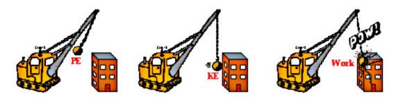
The massive ball of a demolition machine possesses mechanical energy – the ability to do work. When held at a height, it possesses mechanical energy in the form of potential energy. As it falls, it exhibits mechanical energy in the form of kinetic energy. As it strikes the structure to be demolished, it applies a force to displace the structure – i.e., it does work upon the structure.
