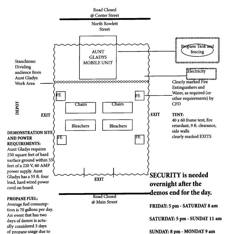
the initial 18 hour start up melt. 250 gallon tank and high pressure regulator supplying 20 psi of
