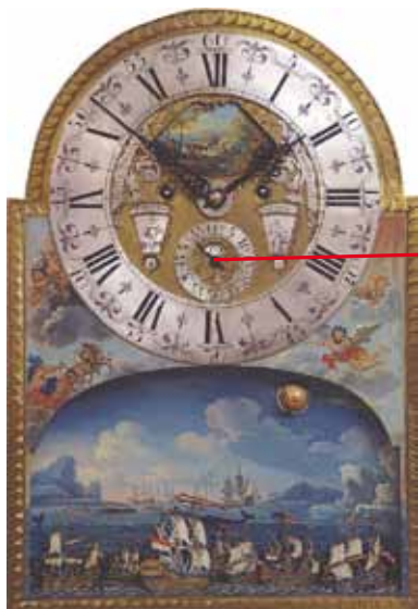
A whaling clock by Pieter Zwaan c. 1750, with rotating spherical moon and seasons aperture below 12 o'clock.
