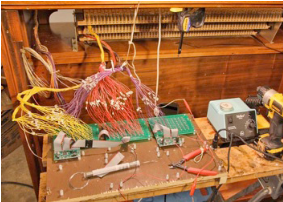
Yes, there are a lot of wires but just connect one at a time. The small boards are the actual midi boards and the larger ones my matrix boards. I did it the hard way - you would not do it this way.
