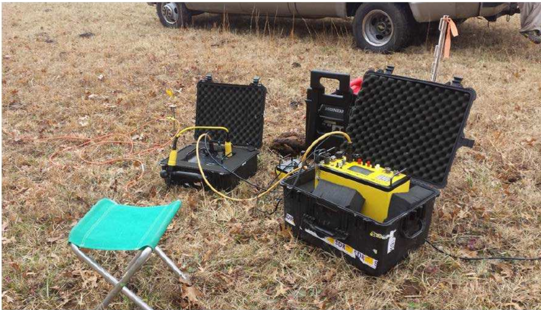
Figure 1 - Electrical resistivity equipment during data collection (12.17.14)
