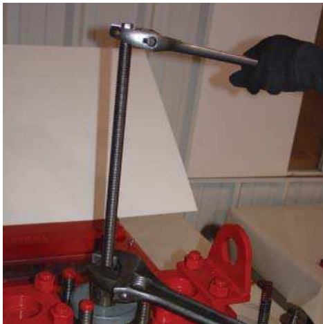
10.) Holding the top of the puller rod in place, tighten the nut until the seat releases.
