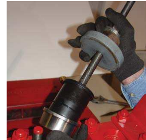
12.) Loosen the puller rod to retract the pins and remove the seat.
