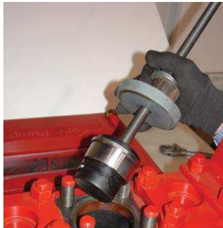
11.) Remove the puller assembly with seat attached.
