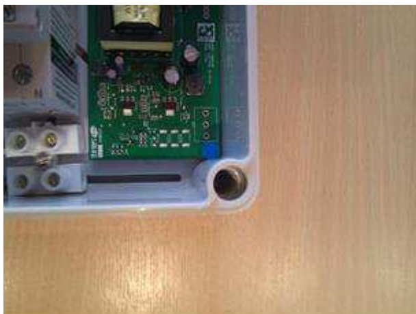
Figure 7. Esprit Intelligent Control Box (v2.0) pre-moulded mounting hole.
