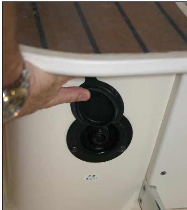
Raw Water Washdown Hose Connection
