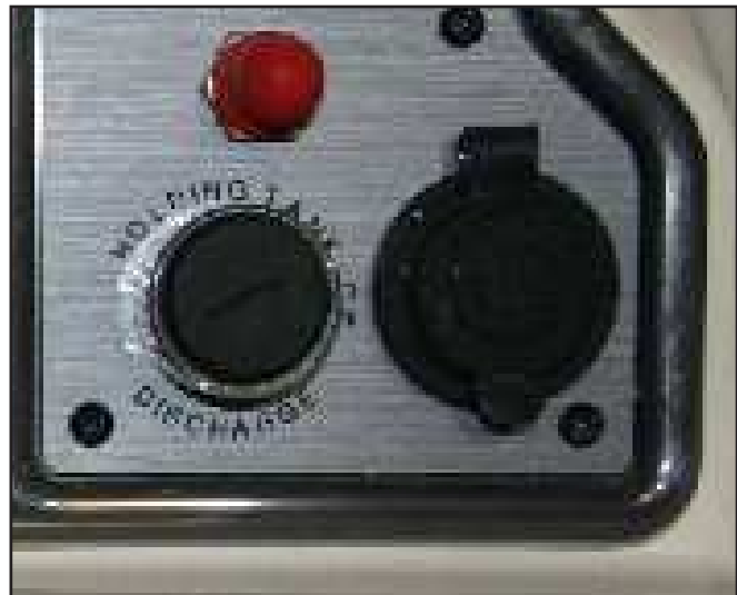
Overboard Discharge Pump Lockout Switch
