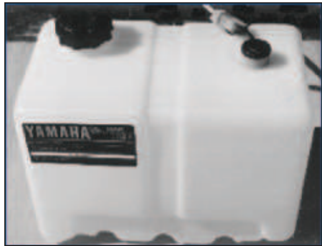
Typical Engine Oil Tank
