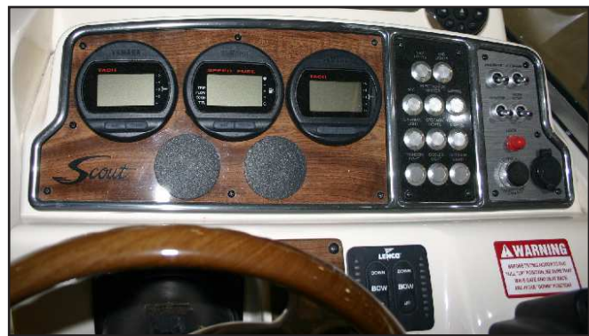
Helm Switch Gauges and Switch Panel
