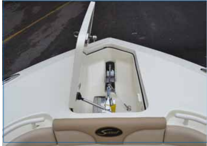
Anchor Locker Deck Hatch
